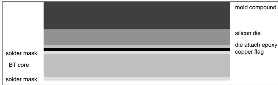
Fig. 3: Schematic of multi-layer model used in PBGA analysis.
