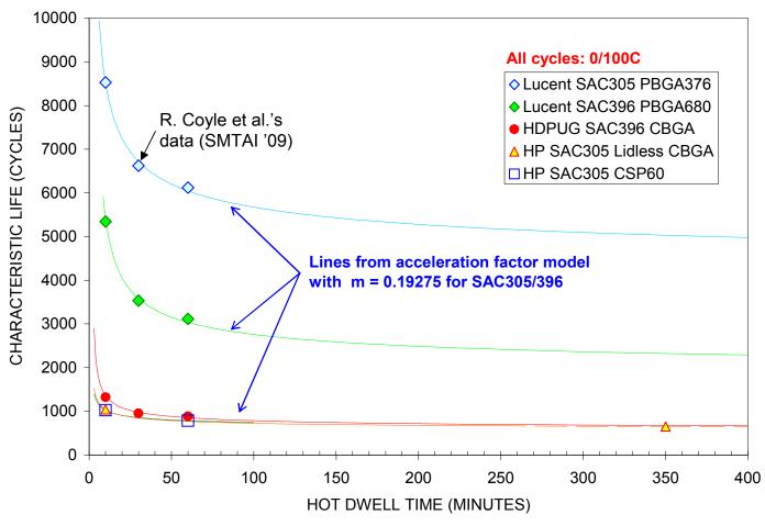
Saturation of cycles to failure with dwell times is more rapid for assemblies with large CTE mismatch
