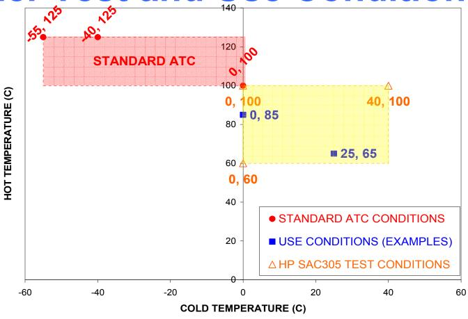
Data are needed for intermediate values of T<sub>min</sub> and T<sub>max</sub> (other than standard ATC conditions) to validate models at temperatures closer to use conditions.
