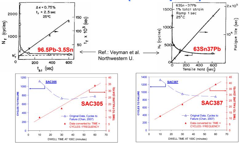
Note: When dwell times are long enough, and within the experimental range, Time to Failure ( $t_f = N_f$  / Frequency) is linear with dwell time.
